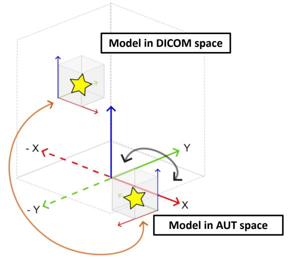
**{bone}-DICOM2AUT.tfm** → Transform between DICOM space and Autoscoper space (orange arrow) **{bone}-PVOL2AUT.tfm** → Transform between world space and Autoscoper space (gray arrow) More Information: <a href="https://autoscoper.readthedocs.io/en/latest/transforms.html">https://autoscoper.readthedocs.io/en/latest/transforms.html</a>
